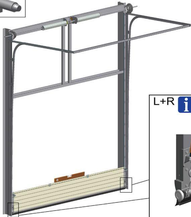
OPTION - cable release switch. Block industrial motor, when cable are released
